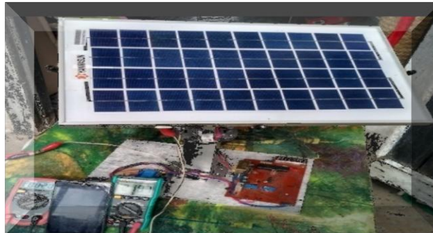
Figure 7 Testing setup for intensity based solar tracking system
